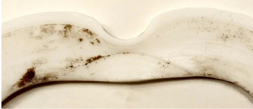
Figure 54: Gasket with Multiple Compressions
