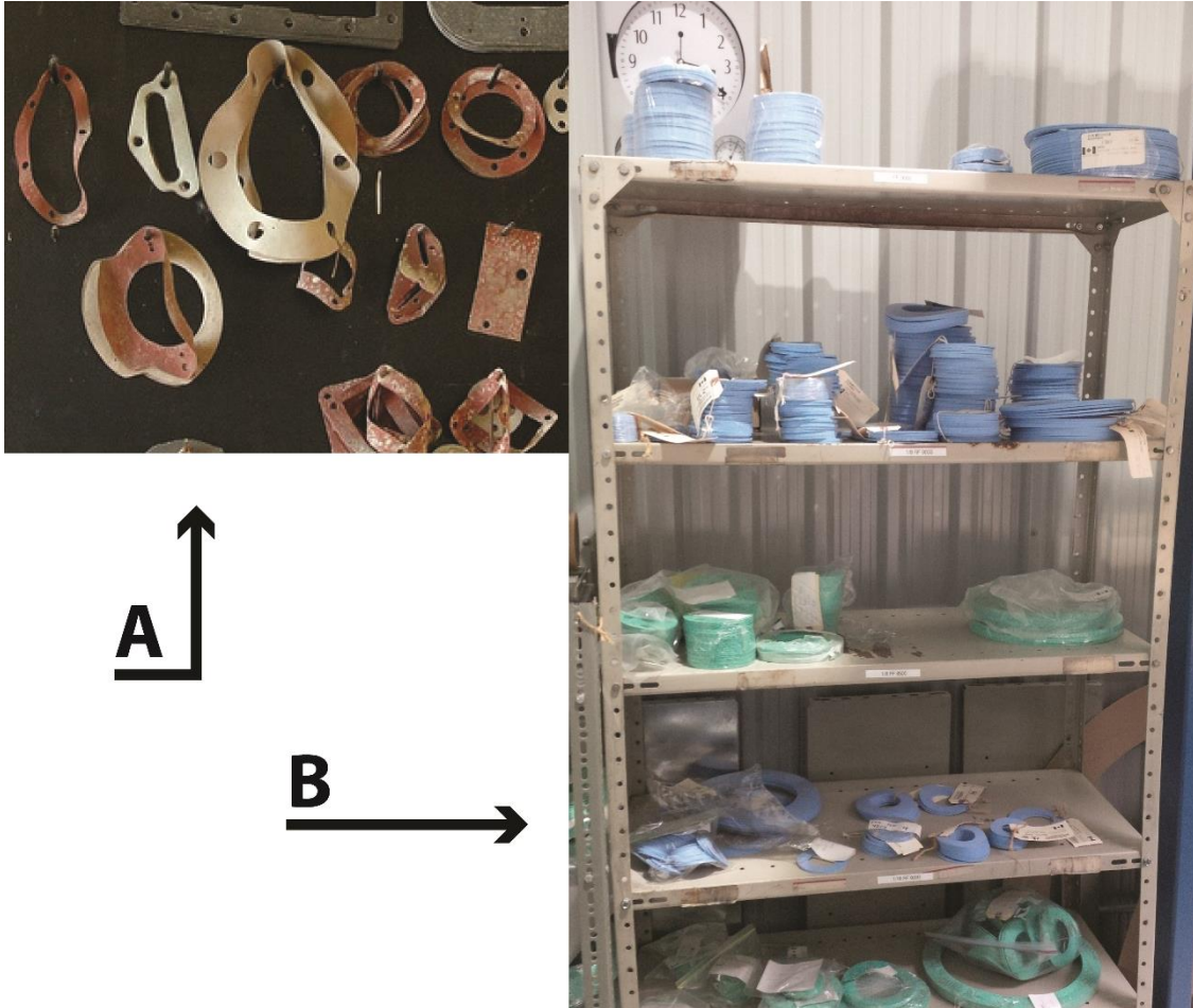
Figure 74: Gasket Storage by Peg Board (A) vs Flat (B)
