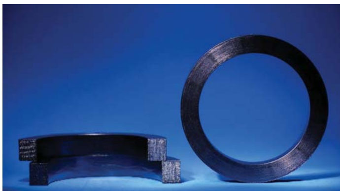
Figure 1: A folded structure in a pure graphite ring and in a metal foil reinforced graphite ring.
