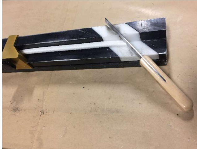
Figure 44. Measuring and Cutting Tool for Compression Packing
