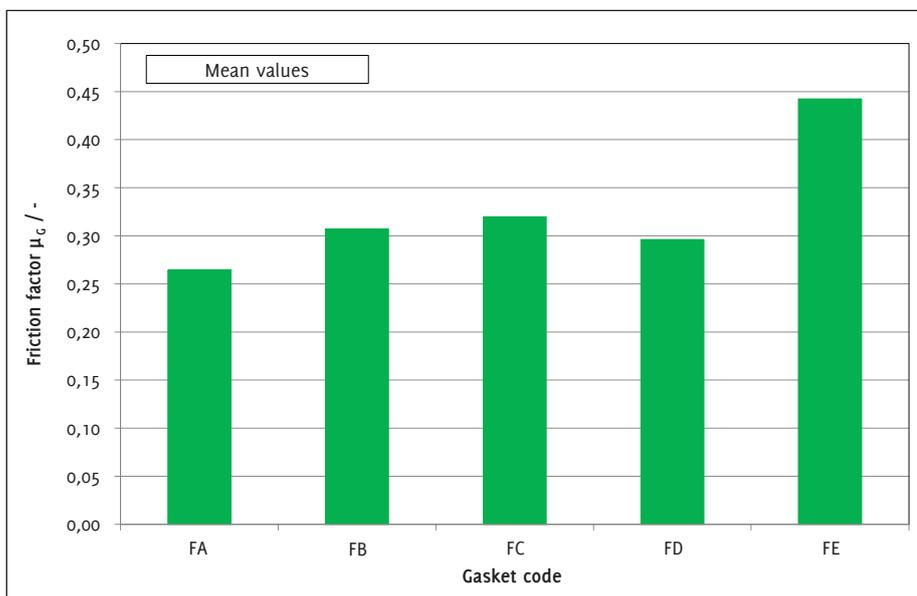
Figure 9: Friction factors for different fibre based gasket materials
