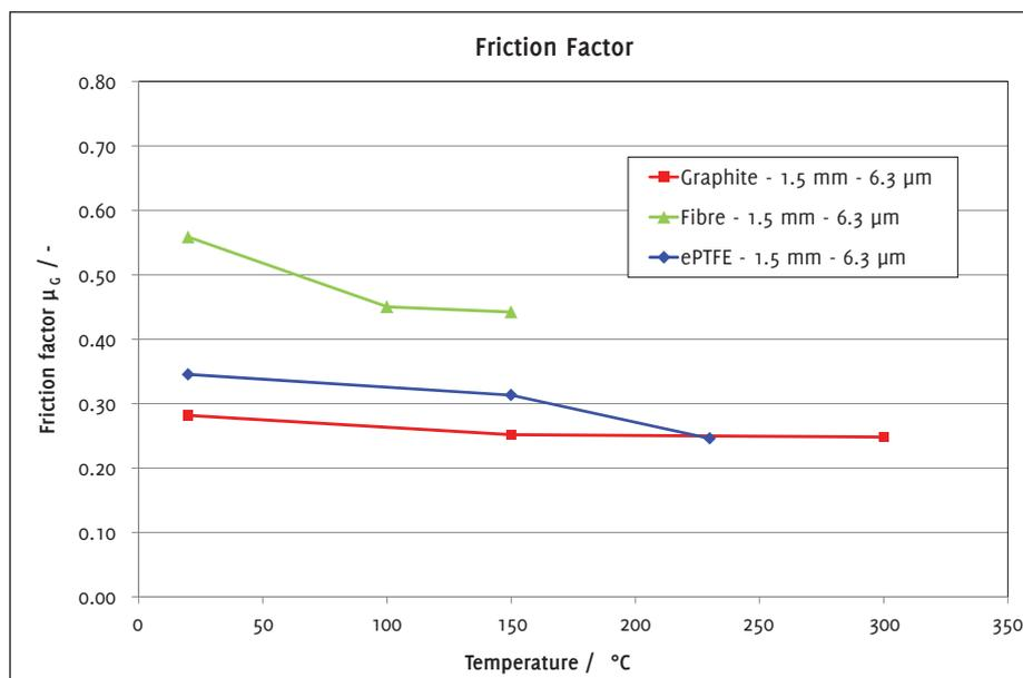
Figure 5: Influence of the test temperature on the friction behavior
