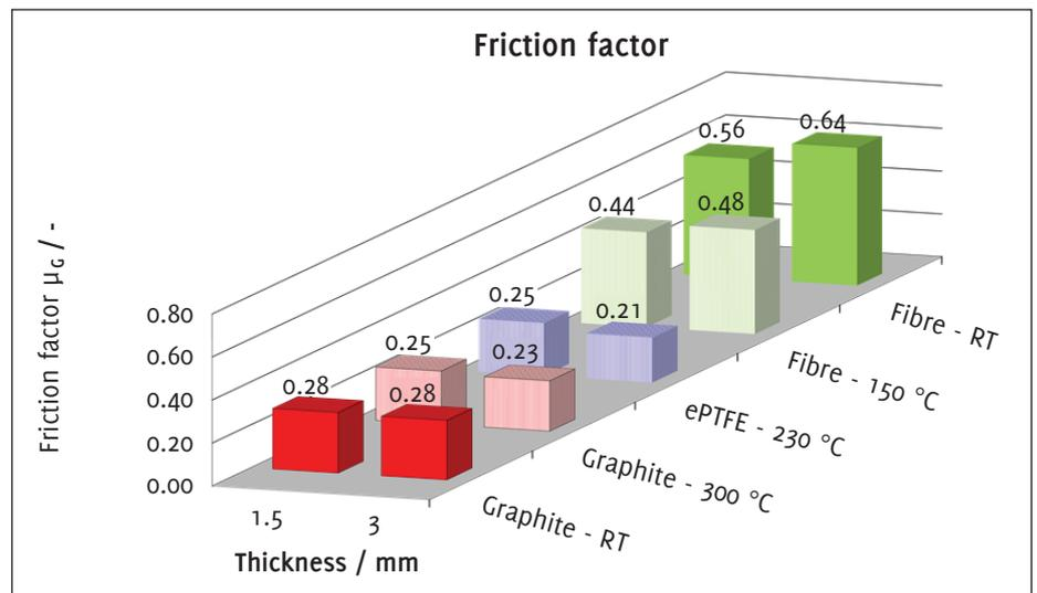
Figure 6: Influence of the gasket thickness on the friction behavior
