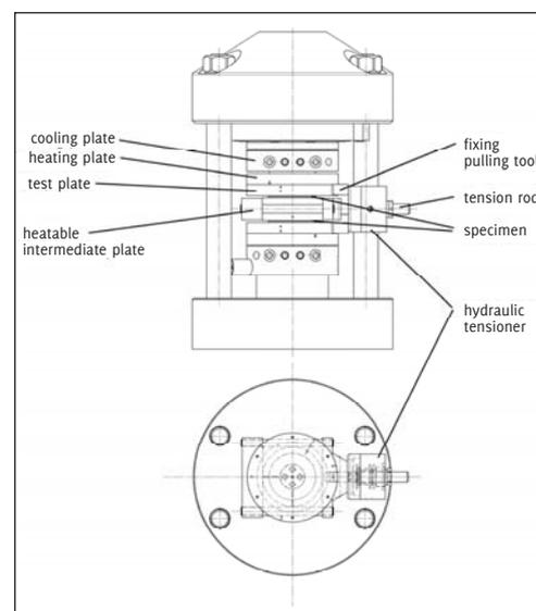
Figure 1: Additional module for friction tests in the testing equipment
