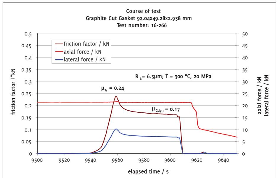
Figure 3: Exemplary course of a friction test
