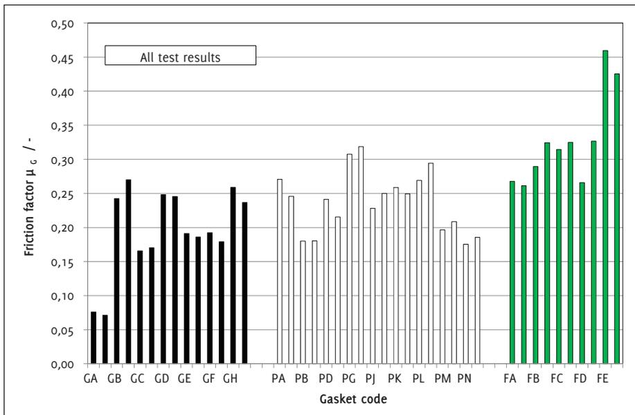
Figure 7: Friction factors for all examined gasket materials (single tests)
