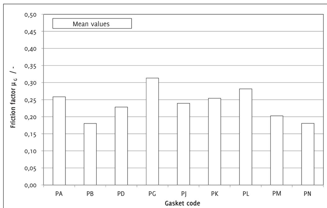
Figure 10: Friction factors for different PTFE based gasket materials
