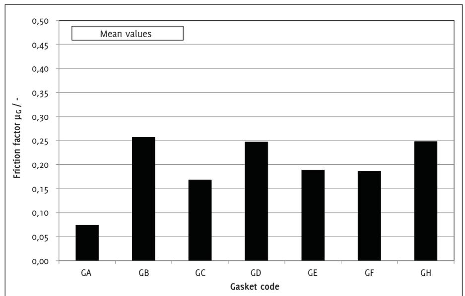
Figure 8: Friction factors for different graphite based gasket materials
