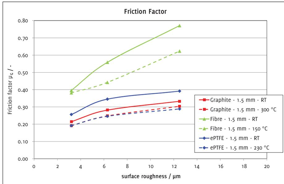
Figure 4: Influence of the flange surface roughness on the friction behavior
