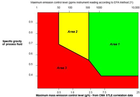
Note: guideline only - emission level will vary with vapour pressure at fluid temperature
