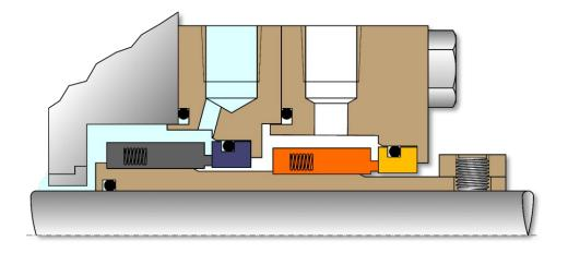
VOC leakage entering the containment chamber between the two seals can then be channeled to a plant flare or vapour recovery system.
