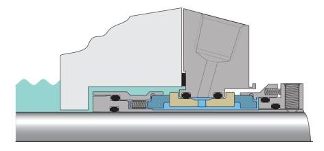
This solution consists of two seals with a barrier fluid (liquid or gas) between them operated at a pressure greater than the process stream. Any leakage (outboard to atmosphere or inboard to the process stream) is of the barrier fluid so selection of a safe barrier fluid compatible with the process stream is essential.
